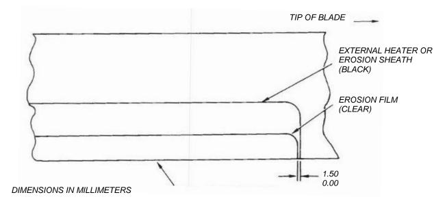
Cut the erosion film to
